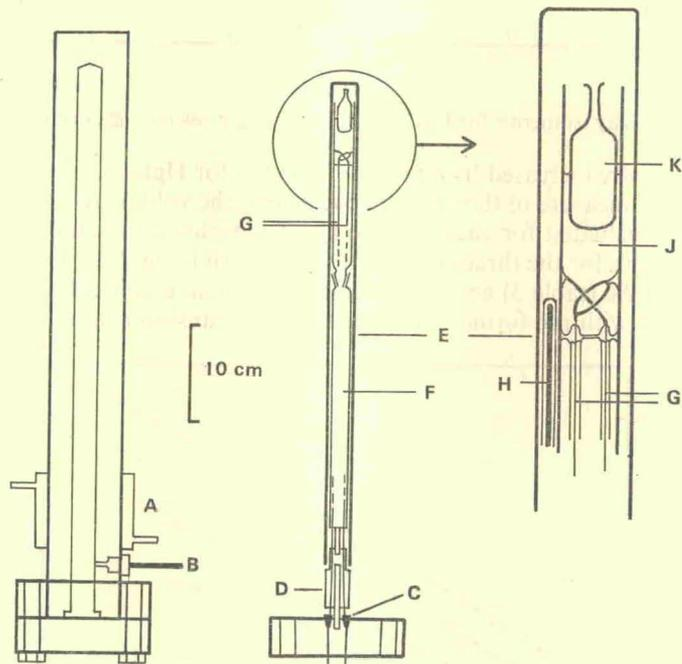
FIG. 2.—Pressure vessel, insert and conductivity cell used for  $\text{HgCl}_2$  and  $\text{HgBr}_2$ . A, water jacket; B, inlet for high pressure gas; C, Bridgman cones for electrical leads to cell and thermocouple; D, pyrophyllite insulator; E, outer glass tube; F, glass column; G, platinum leads, in glass sheaths; H, stainless steel clad thermocouple, in glass sheath; J, melt; K, glass float.
